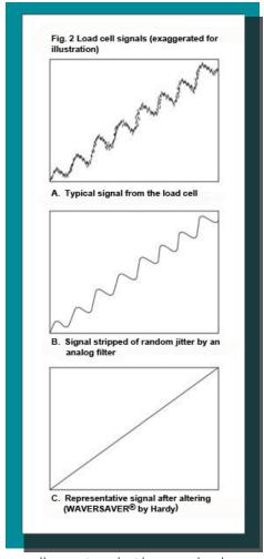
If the signal enters a weight controller equipped with an analog low-pass filter (typically rated from 5 to 20 hertz), the filter will strip off random jitter -- thus providing analog averaging -- and yield a signal similar to that in Figure 2b.
